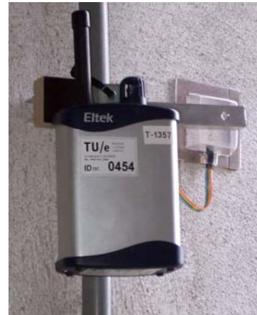
Figure 6. Measurement of the surface temperature and relative humidity at the inside surface of the tower, using a closed box, connected to the inside surface, supposed to be in equilibrium with the wall.
