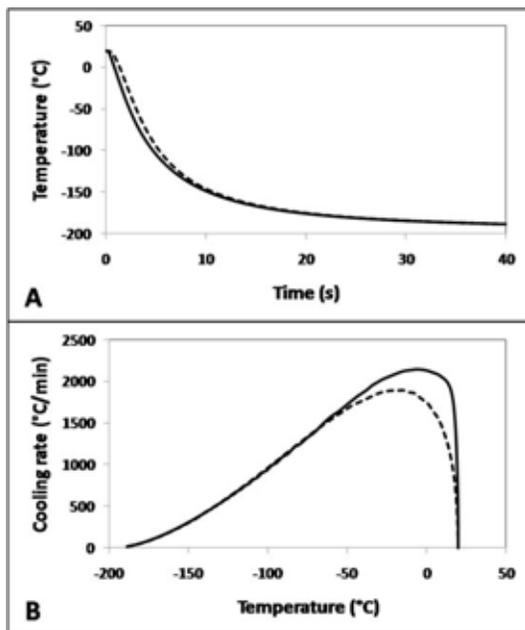
**Figure 3.** Embryo temperature against time (A) and embryo cooling rate against temperature (B) in the Rapid-i for open straw and sealed straw vitrification procedures (solid and dashed lines, respectively).
