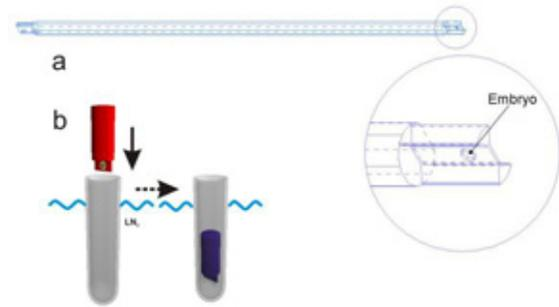
**Figure 1.** (a) A drawing of the Rapid-i stick. The inset shows a detailed view of the holder with a hole for placing the drop of vitrification solution with an embryo. (b) A schematic illustration of the open straw vitrification procedure.
