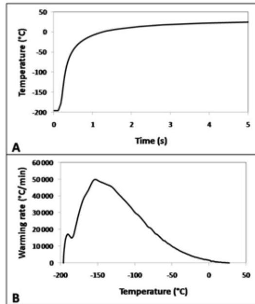
**Figure 6.** Embryo temperature against time (A) and embryo warming rate against temperature (B) in Rapid-i stick warmed in the warming solution.
