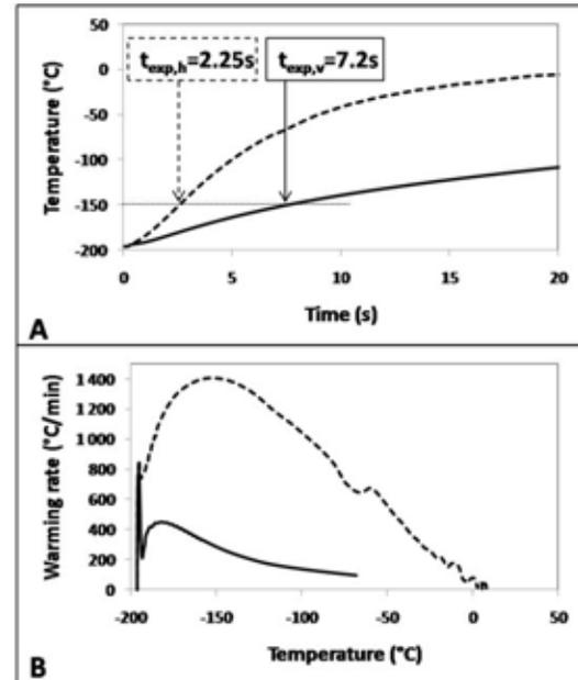
**Figure 4.** Embryo temperature against time (A) and embryo warming rate against temperature (B) in Rapid-i stick when it is exposed to air at room temperature. The stick is held vertically (solid lines) and horizontally (dashed lines).
