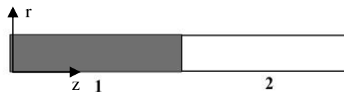
Figure 1. Schematic representation of the computational domain; 1 represents aqueous phase and 2 represents organic phase
