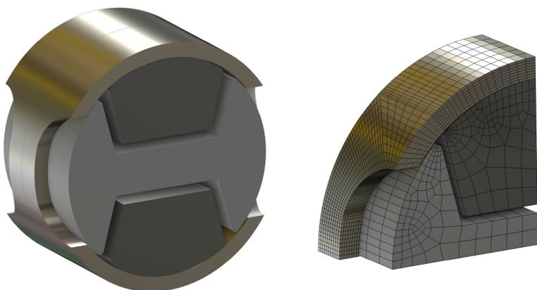
FIGURE 1. Left: The test ring with notches, the bone-shaped center, and the cylinders on which a load is applied (dark gray). Right: 1/8 symmetry is used to save computational time.
