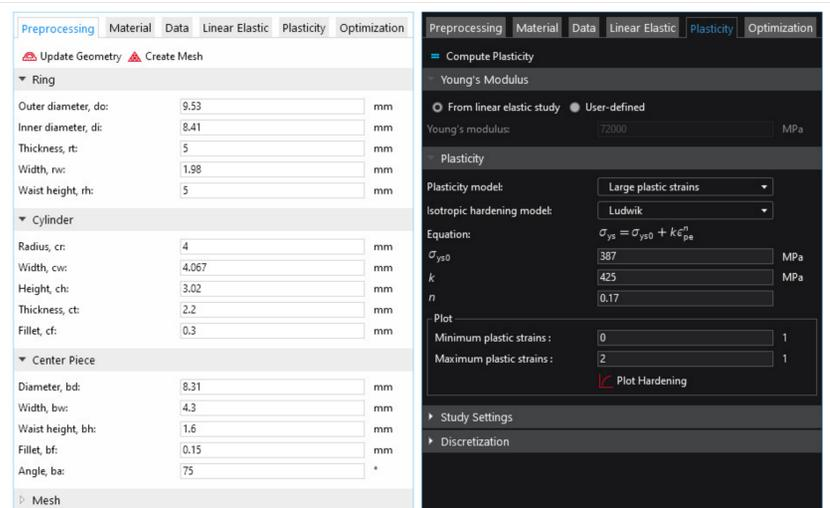
FIGURE 2. Left: Settings for the geometry parameters and the mesh. Right: Plasticity settings in dark theme. The user can choose from 8 different hardening models or specify an analytic hardening function.
