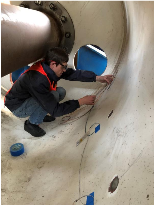
Figure 3. Installation of Strain Gauges Inside the Drum.
