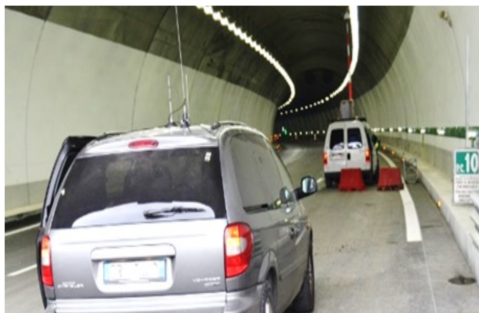
FIGURE 1. Motorway tunnel simulated in COMSOL® and van equipped with antenna system used for reception tests.
