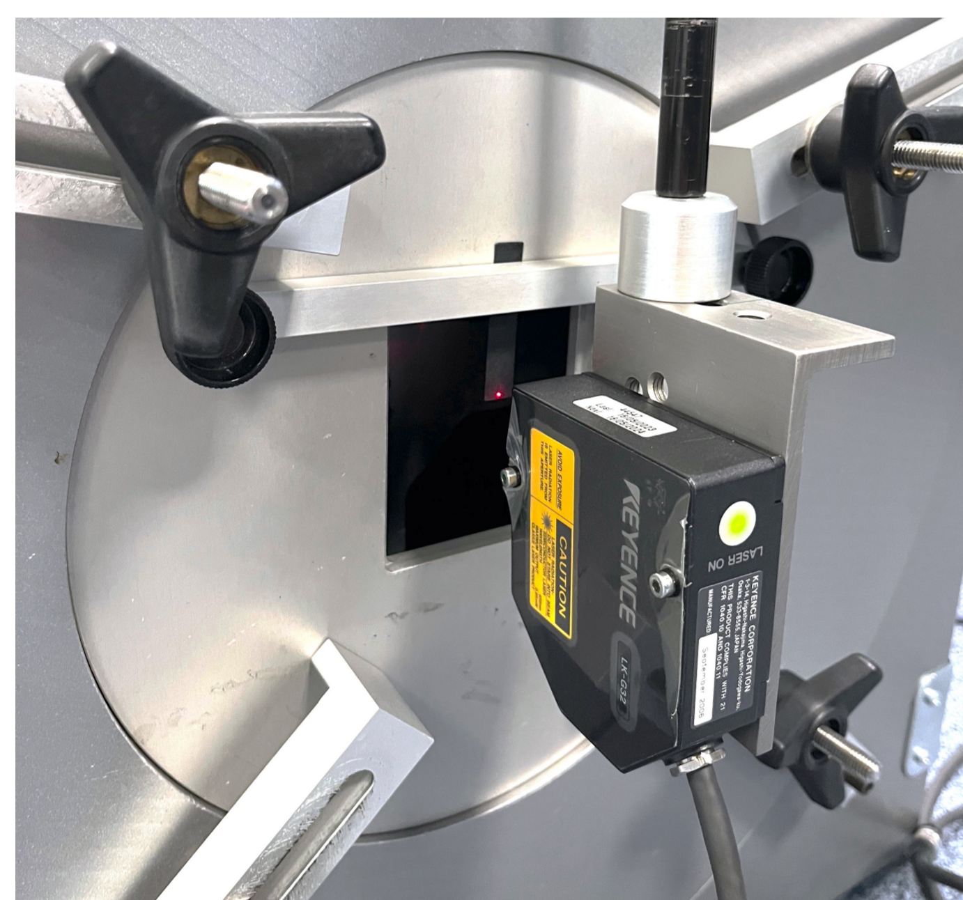
Left: The MPM measurement bench set up for cone material excitation. Right: Simulated excitation used to obtain the material's Young's modulus.
