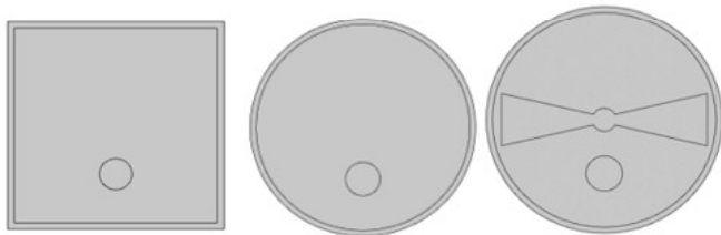
FIGURE 1. 2D models of fermentation trough, dynamic/static cylindrical fermenter and fermenter with propeller.
