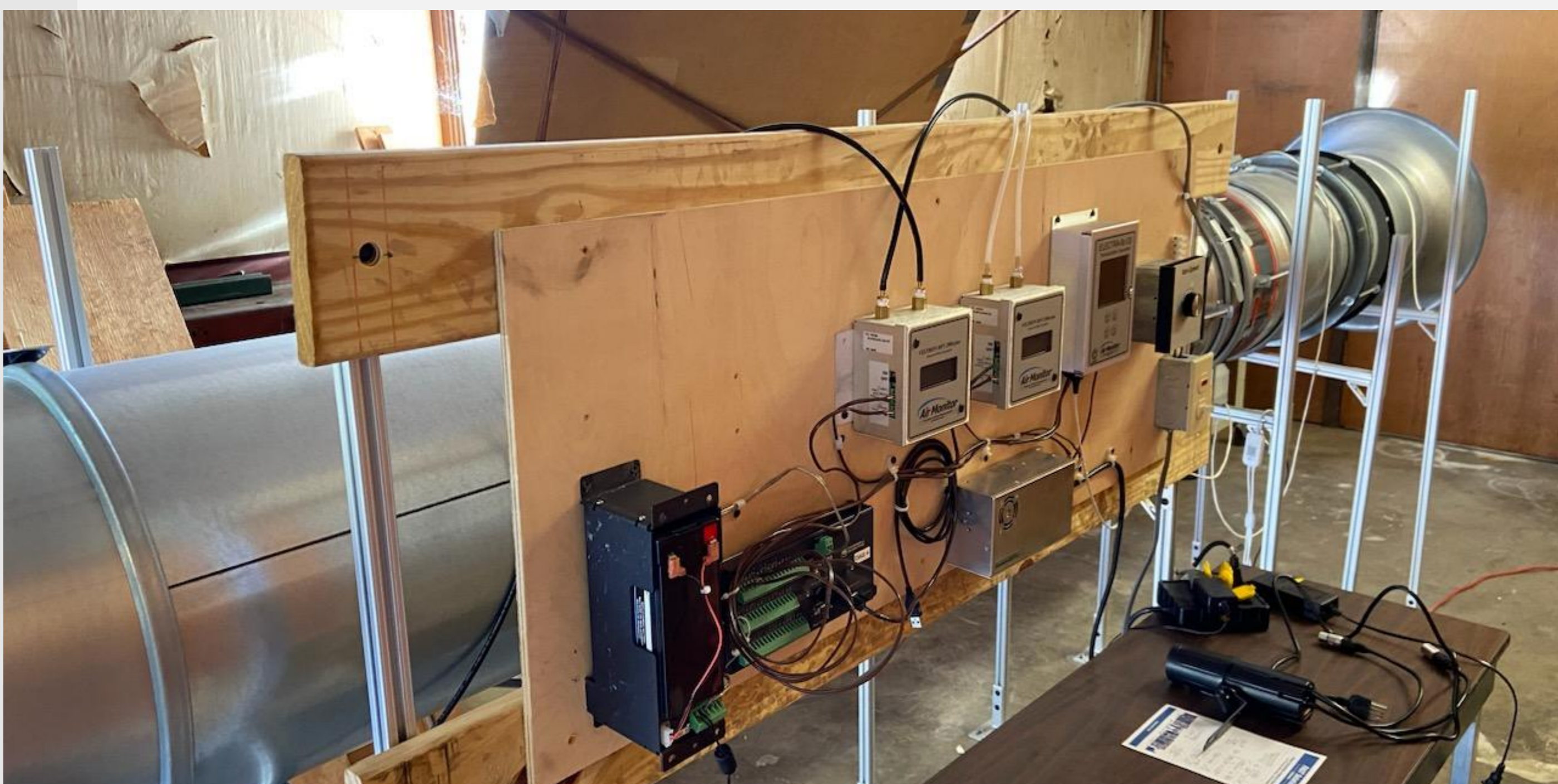
AITF wind tunnel south view showing instrumentation board, cabling, work table, and flow intake within the UT Drive Services Building B structure area.
