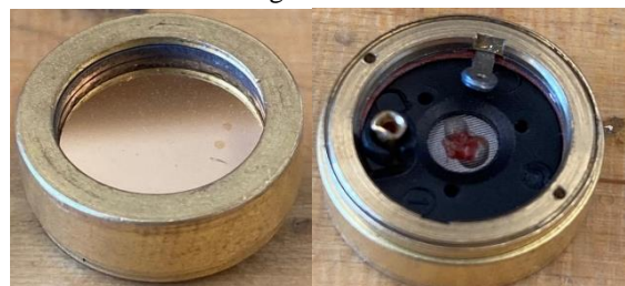
Figure 6: Image of Half Inch Cardioid Cartridge Built and Tested to Validate Model
