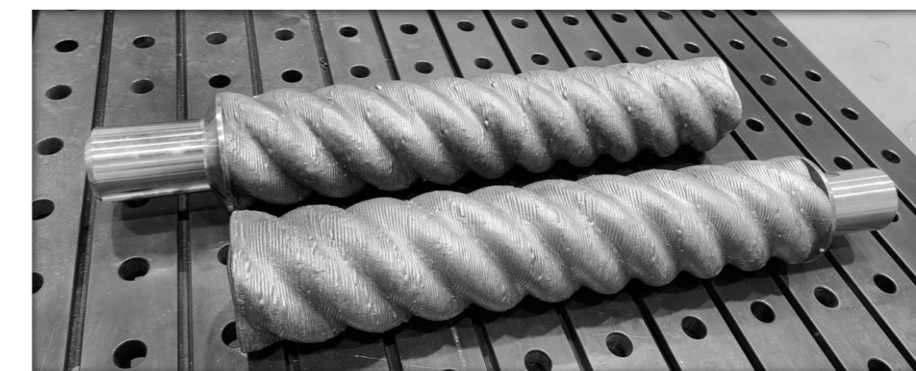
Fabricated part with 60s cooling
