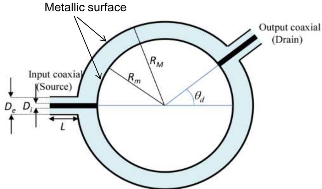
$$D_e = 10 \text{ mm} \quad D_i = 5 \text{ mm} \quad L = 20 \text{ mm}$$
