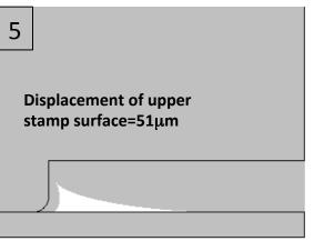
feature height=10  $\mu m$ feature width=20  $\mu m$ thickness of layer above stamp feature=2 mm
