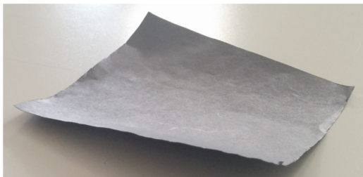
Figure 1. Thermally conductive compound used on transducer prototype.
