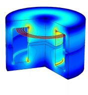
**Figure 1**: The Comsol AC/DC module has been used to analyze a magnetic flux density in the planar transformer core and the current density in the windings
