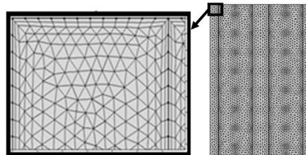
Figure 4. Discretization of the computational domain. The example refers to the case of empty channels.
