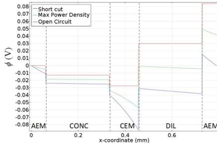
**Figure 7.** Potential profile within the cell pair with empty channels, fed by 4M-0.5M solutions at 1 cm/s, at different external loads.  $R_{blank}$  was set equal to zero in order to visualize inside the cell pair all the internal loss. The values are taken along a horizontal midline.
