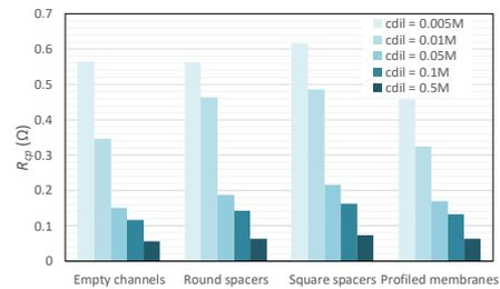
**Figure 9.** Cell pair resistance for different dilute concentrations and membrane/channel configurations, at the fluid velocities that maximize the net power density, and with 4M concentrate solution.
