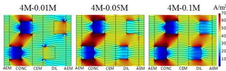
**Figure 8.** Current density distribution within the cell pair with profiled membranes, fed by 4M concentrate solution and various dilute solutions at 1 cm/s. Simulations at maximum  $P_{d,gross}$  conditions.
