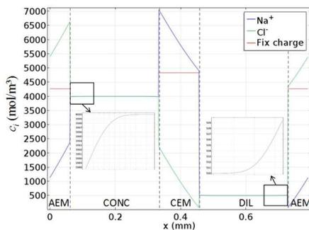
**Figure 6.** Concentration profiles within the cell pair with empty channels, fed by 4M-0.5M solutions at 1 cm/s. Simulation at maximum gross power density conditions ( $R_{ext} \approx 2 \Omega$ ). The values are taken along a horizontal midline.
