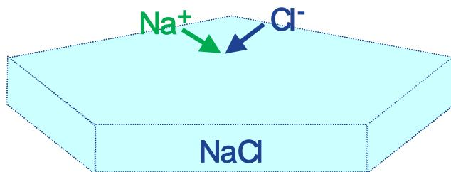
$\text{NaCl}$  crystallization from solution: 1<sup>st</sup> order in  $[\text{Na}^+]$  and  $[\text{Cl}^-]$
