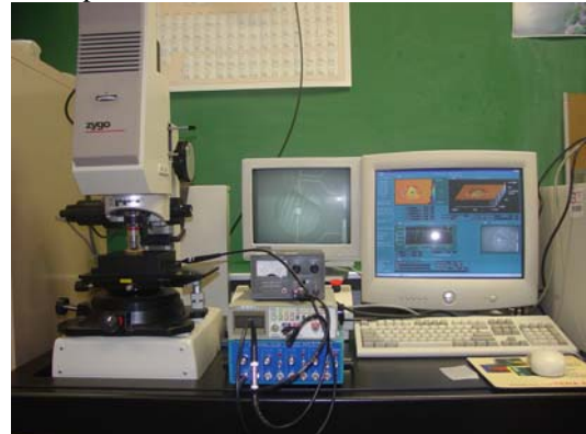
Figure 6. Static Deflection Measurement Setup
