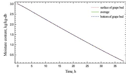
**Figure 3.** Evolution of grape moisture content during the drying process.
