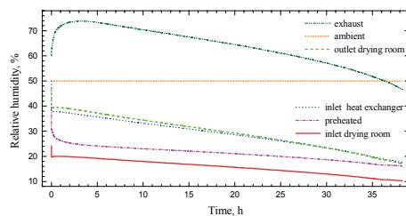
**Figure 5.** Relative humidity of drying air at different locations vs. drying time.
