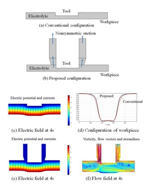
Figure 1: Propsed electrochemical machining and computational results.
