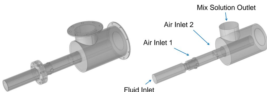
Figure 2. Foam Chamber CAD Model
