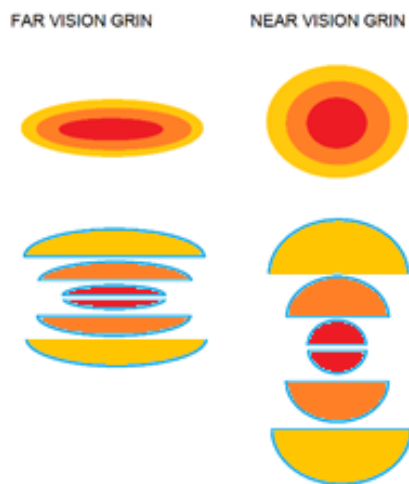
Figure 14: Simplified finite multilayer representation of the GRIN with decomposition in equivalent lens for each layer.
