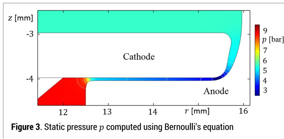
Figure 3. Static pressure  $p$  computed using Bernoulli's equation
