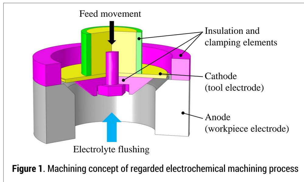
Figure 1. Machining concept of regarded electrochemical machining process
