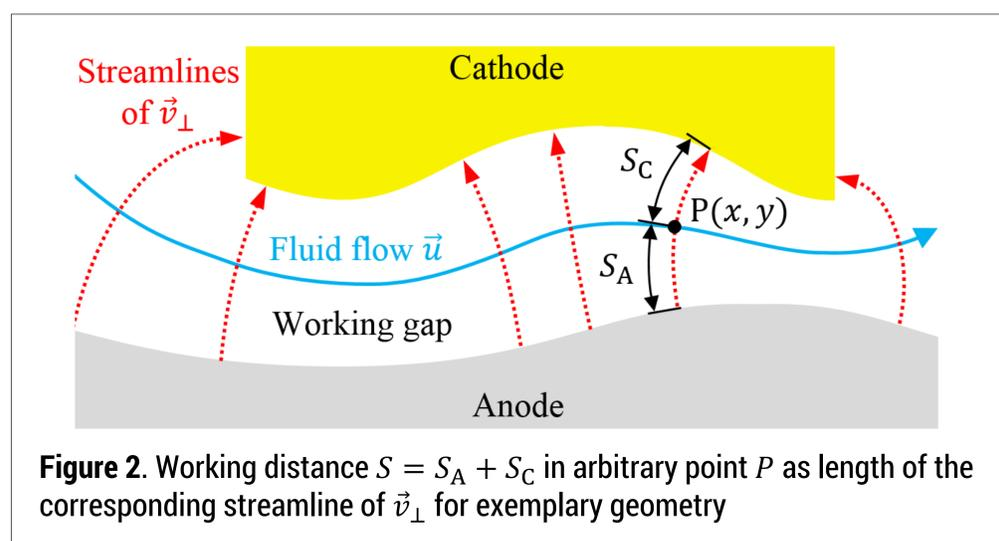
Figure 2. Working distance  $S = S_A + S_C$  in arbitrary point  $P$  as length of the corresponding streamline of  $\vec{v}_\perp$  for exemplary geometry
