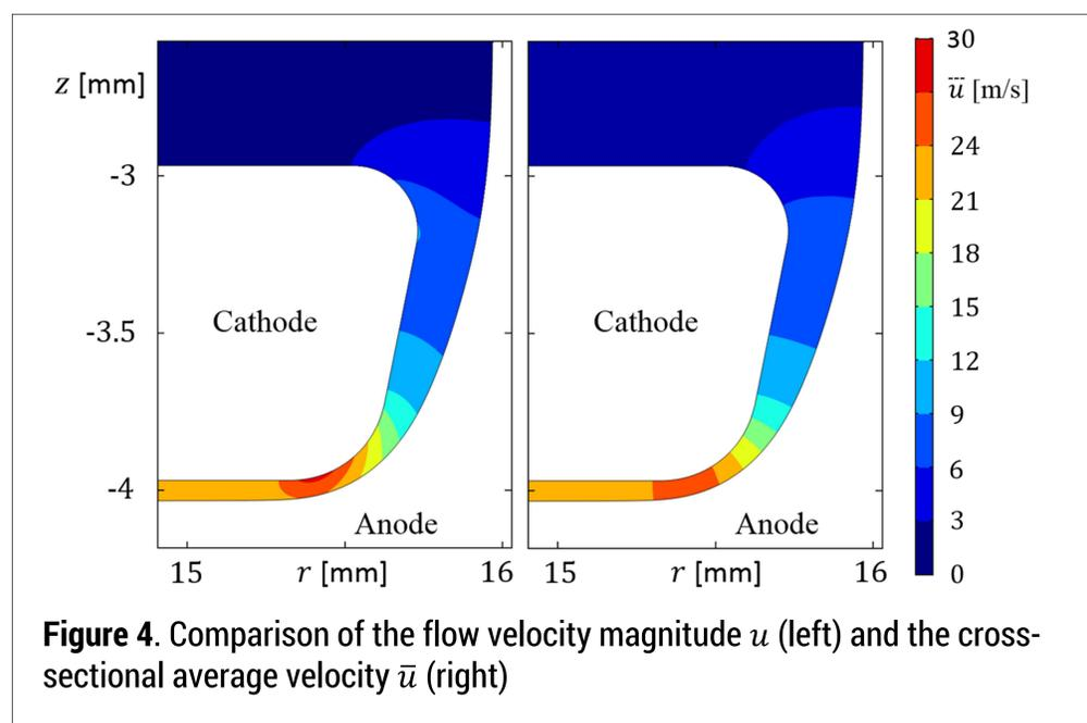
Figure 4. Comparison of the flow velocity magnitude  $u$  (left) and the cross-sectional average velocity  $\bar{u}$  (right)
