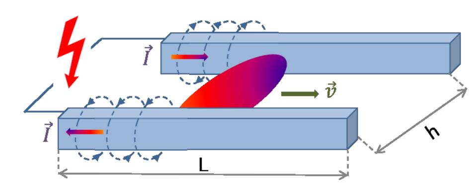
In case of a fault, an electric arc takes place and propagates along the electrodes.
