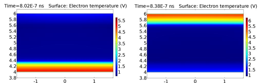
Figure 3. Electron temperature distribution during half period.
