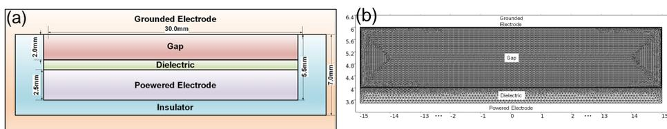
Figure 1. (a) Plasma source geometry and (b) Model in COMSOL
