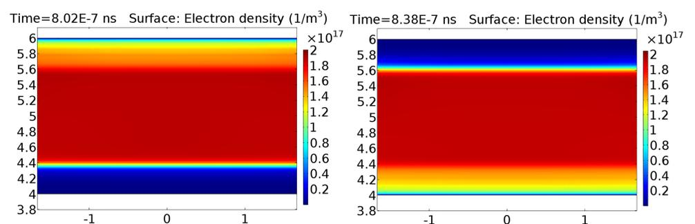
Figure 2. Electron density distribution during half period.
