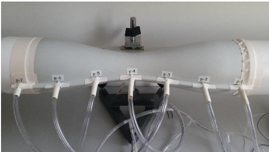
Figure 3. Venturi tube with connected pressure measuring pipes
