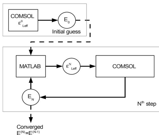
Illustration 4: Schematic of the iterative procedure, as it has been implemented using COMSOL for the solution of the wave equation and MATLAB for the evaluation of the effective local damping term  $\bar{\epsilon}_{\text{ELDeff}}^{(N)}$
