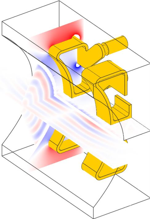
Illustration 5: Snapshot of the right hand polarized electric field of the ICRF waves as they are radiated from the antenna and they propagate in a section of the Alcator C-Mod tokamak.
