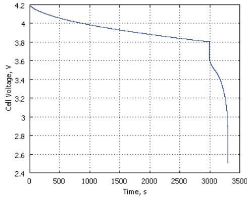
**Figure 8.** Cell Voltage at C/2 discharge for 3000s followed by a 3C pulse discharge
