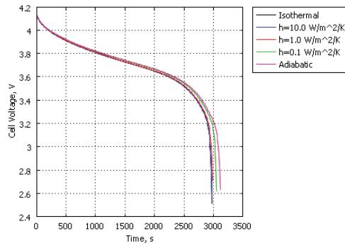
**Figure 5.** Cell Voltage for 1C discharge process under different cooling conditions
