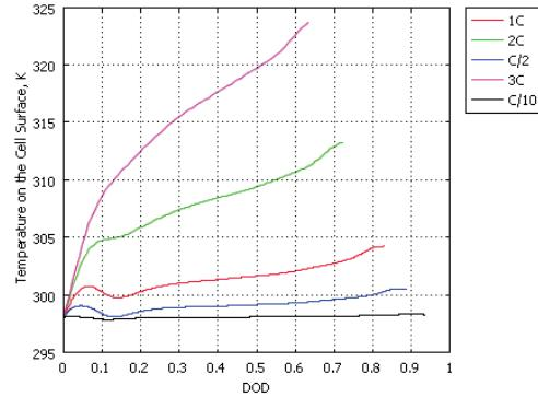
**Figure 7.** Temperature on the cell surface during discharge process under different current rates while the heat transfer coefficient  $h=1.0 \text{ W/m}^2/\text{K}$  where the DOD is defined as:  $\text{DOD} = \text{time} * \text{C rate} / 3600$
