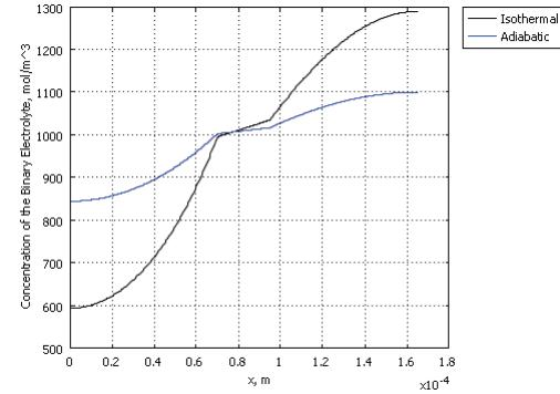
**Figure 6.** Comparison of the concentration profiles of the binary electrolyte at the end of the 1C discharge process under the isothermal condition and the adiabatic condition
