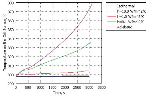
**Figure 4.** Temperature on the cell surface during 1C discharge process under different cooling conditions
