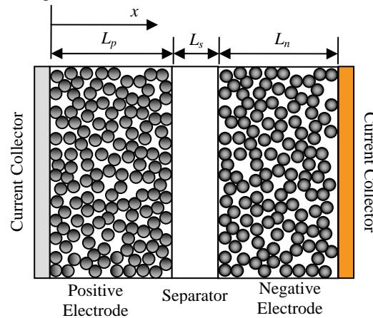
**Figure 1.** Schematic of a Lithium ion battery
