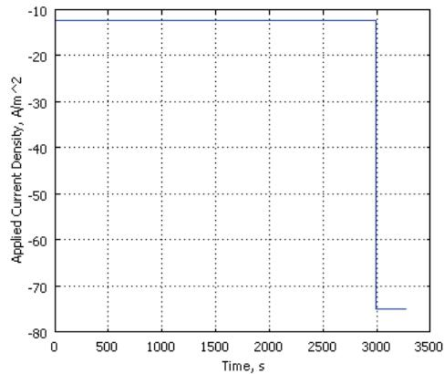
**Figure 3.** Current density profile in the discharge process including a 3C pulse
