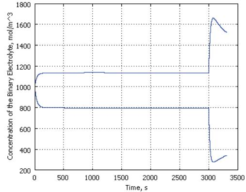
**Figure 10.** Concentration of the binary electrolyte at the two ends of the cell (the bottom line is at  $x=0$ , the top line is at  $x=1.65e-4$ ) in the C/2 discharge process with a 3C pulse
