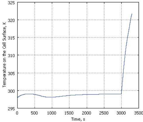
**Figure 9.** Temperature on the cell surface in the discharge process with 3C pulse
