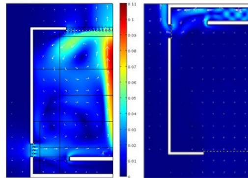
**Figure 4.** Proposed package simulation results for face up and face down orientations: Arrow and color scale indicate air speed direction and value (m/s)
