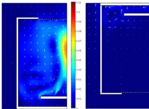
**Figure 2.** Standard package simulation results for face up and face down orientations: arrows and color scale indicate air speed direction and value (m/s)
