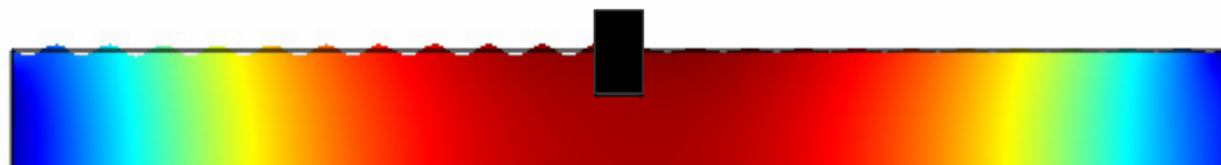
Fig 4. The 2nd order low frequency potential \Phi_{wLF}^{(2)} in color scale, and elevation due to high & low frequencies components (2nd order wave correction and scattered), solving Fig 1. Vertical deformation = 1.
