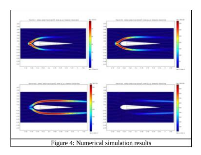
Surface plots of the investigate model shown in Figure 4 display, in the sequential images, the movement of the charge inside of the duct. We can observe the charge flow is spit in two currents one having an excess of positive charge, the other one negative charge. The calculation of the inductive electromotive force has been obtained by considering an equivalent circuit where the primary winding is due to the
