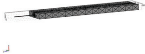
Figure 5 - Geometry of the Bragg grating fiber optic embedded composite material. The COMSOL mesh grid can be observed.
