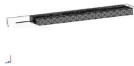
Figure 2. Geometry of the Bragg grating fiber optic embedded composite material. The COMSOL mesh grid can be observed.
