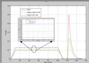
Using simulations we have seen that the concentration factor improve 1.78 times. Experimentally, we have obtained an improvement of 1.85 factor. This value is really near to our simulations and it validate this.
