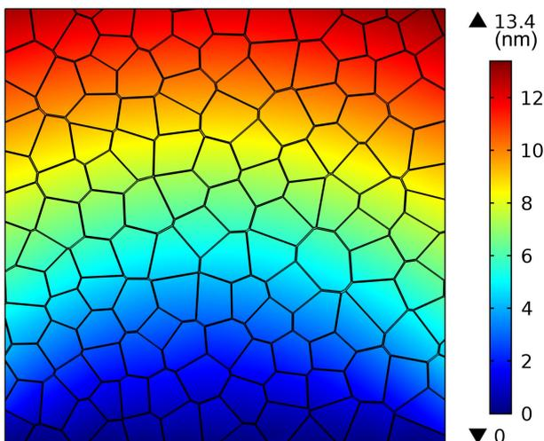
**Figure 1:** Displacement field distribution of piezoelectric composite under the applied electric field ( $E$ ) of 2 kV/mm.
