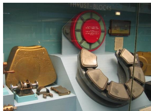
Figure 3. Michell thrust block at the London Science Museum (By Andy Dingley - Own work, CC BY-SA 3.0, https://commons.wikimedia.org/w/index.php?curid=4944466 )
