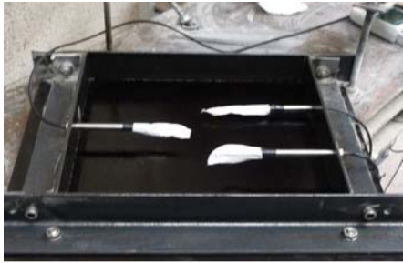
Figure 2. Instrumentation of the slab.
