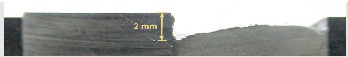
Photograph after cross-sectional cut of AE44 – MS couple after 3 days of immersion Comsol Conference, Bangalore, October 29 - 30, 2010
