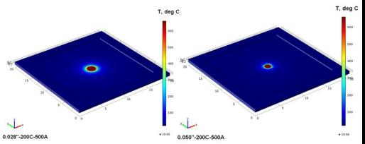
Damage areas & simulated final T-distributions. The red areas are the damage as a result of 200 C at 500 A.
