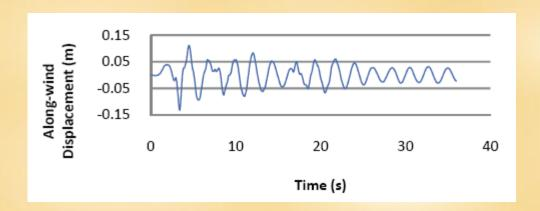
The displacement varies mostly at the first tower bending frequency (0.46 Hz) but has some higher-frequency components
