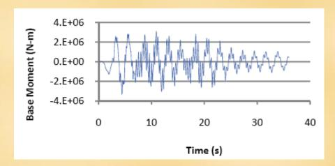
The bending moment time-history displays more content at frequencies higher than the first natural tower bending mode
