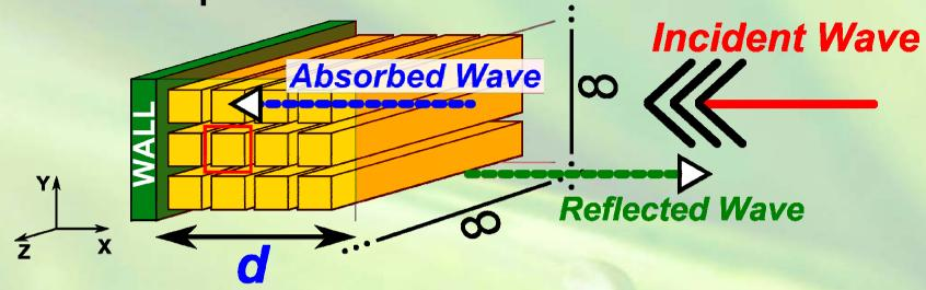
$$H = \left(\frac{\frac{-2i\omega d}{c_{eff}}}{1 + e^{\frac{-2i\omega d}{c_{eff}}}}\right) = \operatorname{cotanh}(iQd)$$
