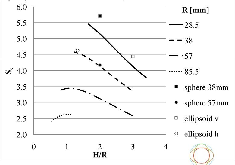
Normalized coefficient  $k_N$  in function of H/R ratio for different shield shapes (same thickness 0.5mm and  $\mu r$  550 for all shields)
