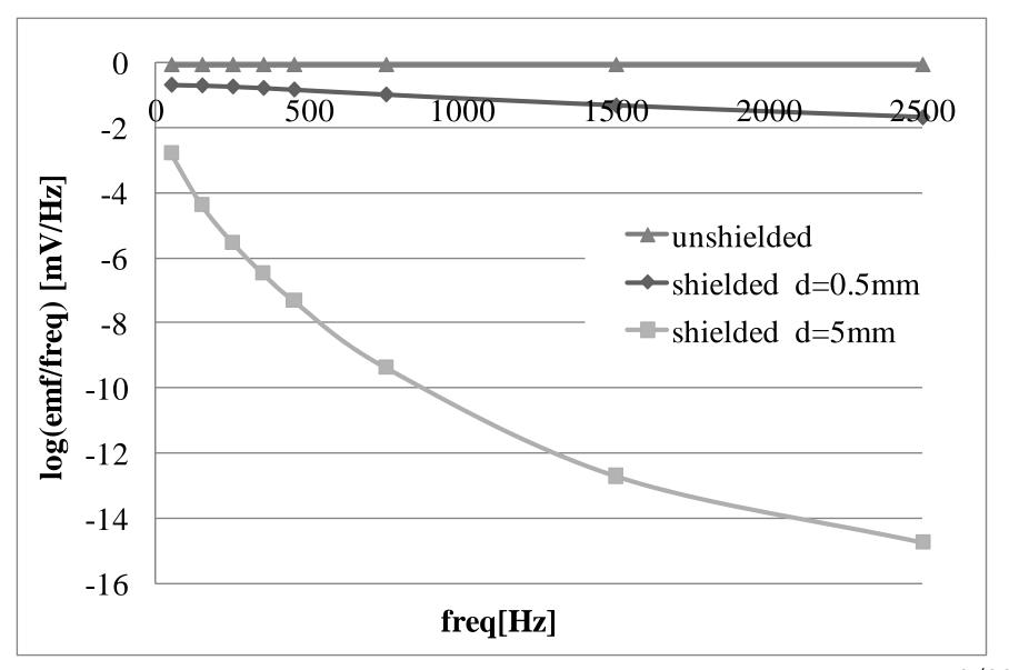
Shield shape influence on transformer linearity coefficient as function of frequency of input signal on primary winding
