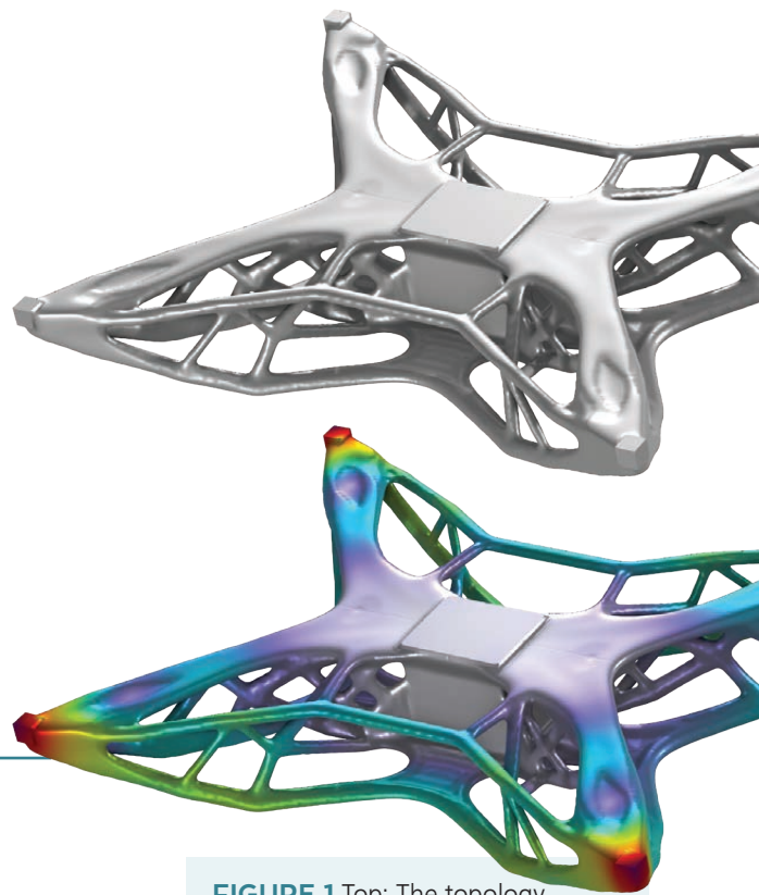
FIGURE 1 Top: The topology optimization functionality in COMSOL Multiphysics® with the add-on Optimization Module can be used to generate a drone model with good performance. Bottom: The model is shown with the displacement magnitude to help us visualize the optimization process.
