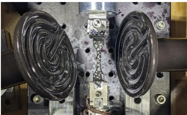
FIGURE 4 This experimental setup features a tensile test of the lithium (center, black with silver dots) between two black ceramic heaters.
