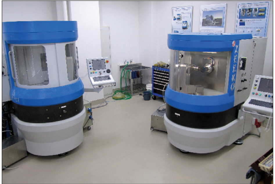
Figure 2: The Zeeko Intelligent Robotic Polisher. The position and pressure of the FJP tool are controlled by the Zeeko 7 axis CNC (Computer Numerical Control) machine tool controller.
