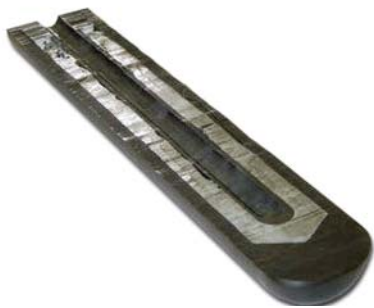
FIGURE 1: Cross-section of a typical fixed-point cell showing the graphite container, the metal ingot, and the central well for insertion of the thermometer.
