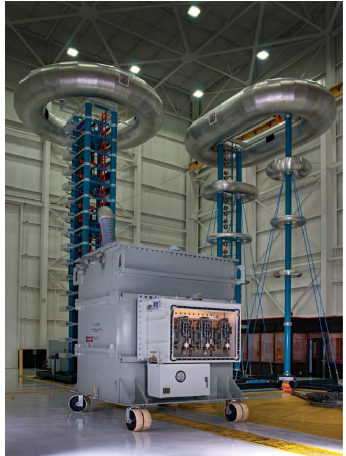
Vacuum Reactance Load Tap Changer at ABB's Alamo, Tennessee Facility.
