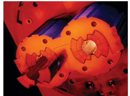
Figure 2. Detail of the main dipole aperture. The superconducting coils are kept in place by means of austenitic steel collars to counteract electromagnetic forces of 2 MN/m per coil quadrant at nominal field.
