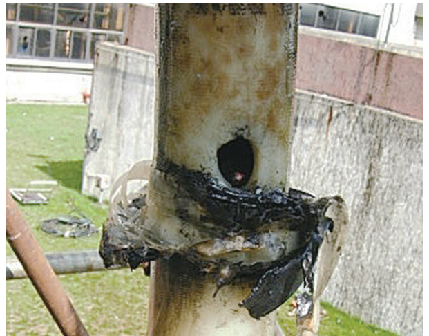
Figure 2. Left: Water tree caused by the interaction between the electric field and moisture. Right: Close-up of the mechanical damage to the insulation layer.
