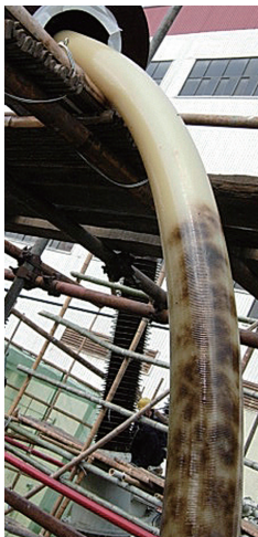
Figure 2. Left: Water tree caused by the interaction between the electric field and moisture. Right: Close-up of the mechanical damage to the insulation layer.
